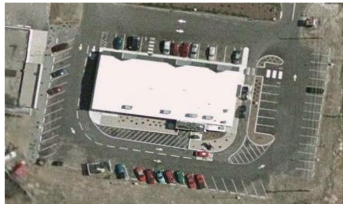
The above image shows a drive-up lane circling the building, separated from parking access. (Image capture from Google Earth)
