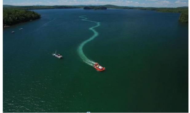
A large barge is used to conduct an aluminum treatment at upstream East Pond to address chronic internal P loading. (Photo credit, 7 Lakes) Alliance)
